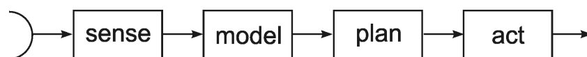
Fig. 16.1 Schematic presentation showing how in an animal or an artificial system the sensory input may cause a behavior action
